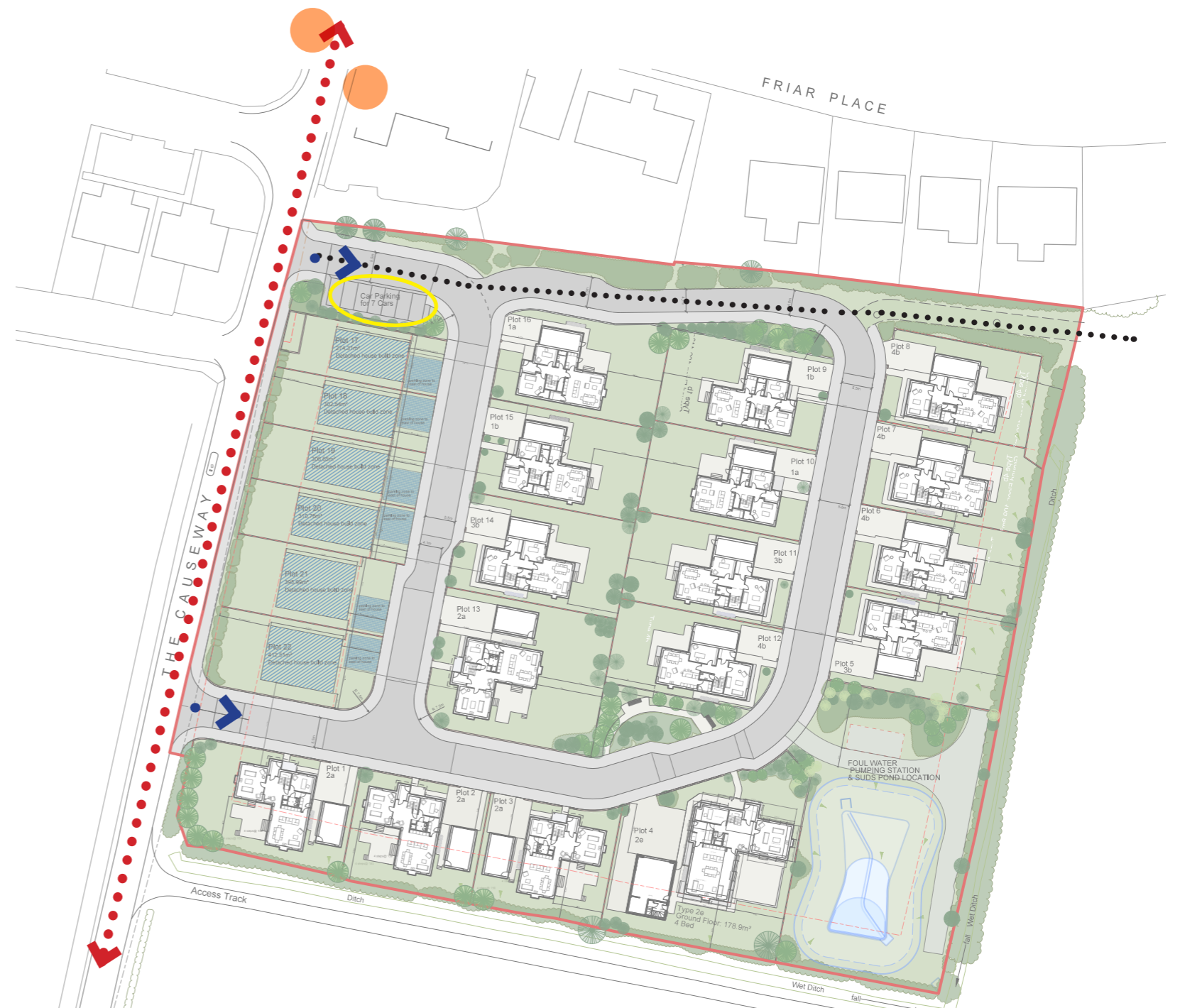
A / Site Plan Showing Accessibility and Connections
